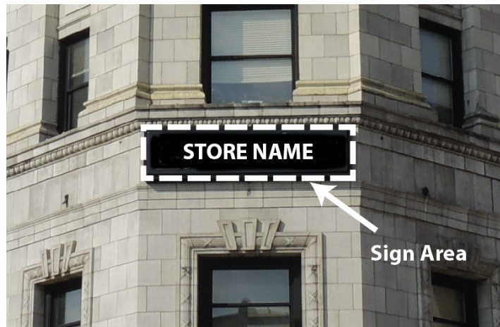
Figure C: Illustration of computing the sign area for wall signs with a background panel or cabinet.
