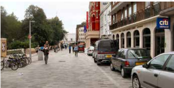
Shared streets are narrow ways designed for use by pedestrians, cyclists and motorists. They do not have raised curbs and feature pavers to slow vehicles.
