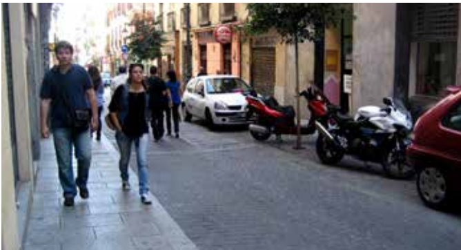
Shared streets are narrow ways designed for use by pedestrians, cyclists and motorists. They do not have raised curbs and feature pavers to slow vehicles.
